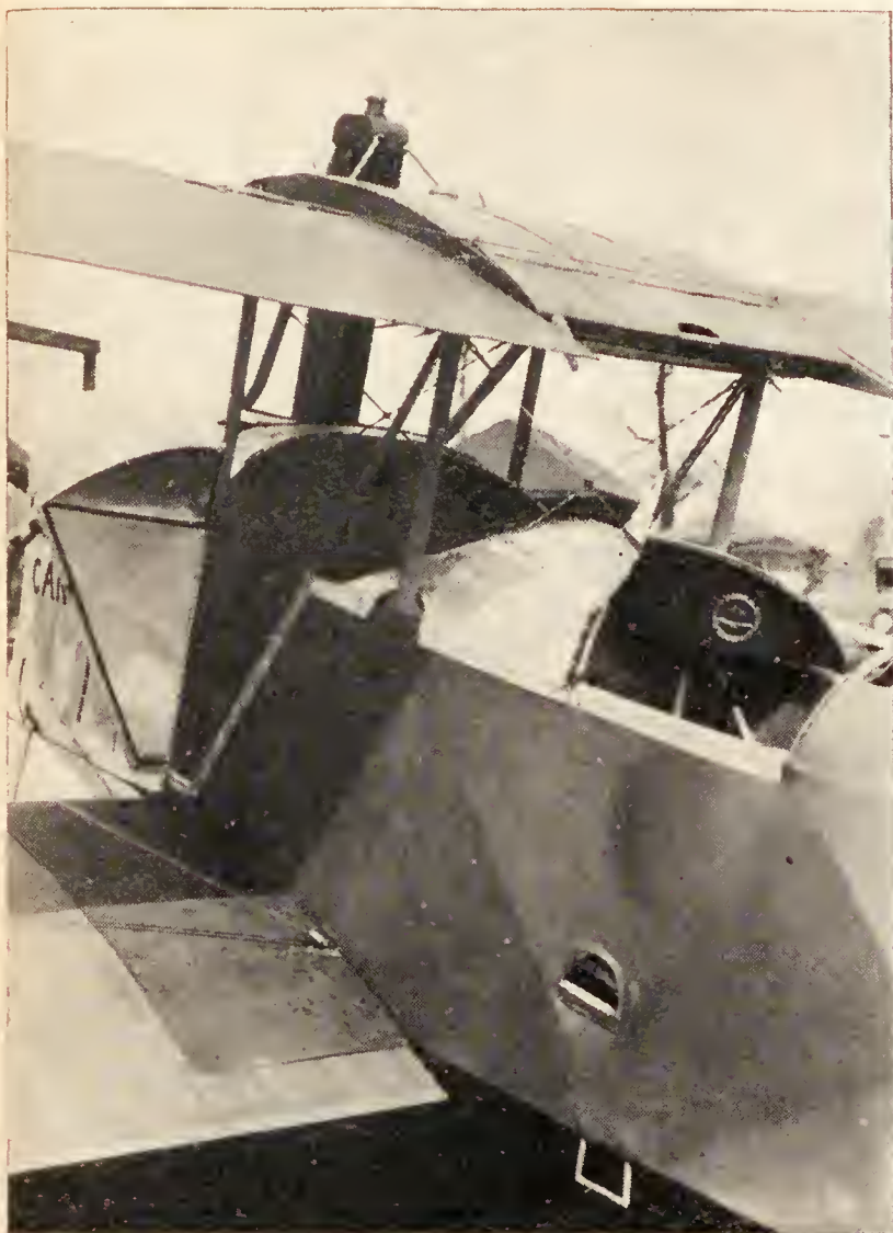
A close-up view of the "Canary," showing the easy access to the passenger compartment to the front of the pilot's cockpit. This is a special feature of this very promising ship.
